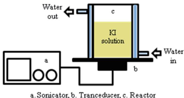
Fig. 1 The schematic experimental set up.
