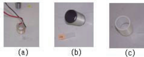
Fig. 2 Photographs of the actuator(a), carbon sensor(b) and teflon sensor(c)
