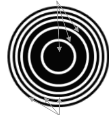
Fig. 1 Illustration of the new annular array pattern (a case with 6 elements).
