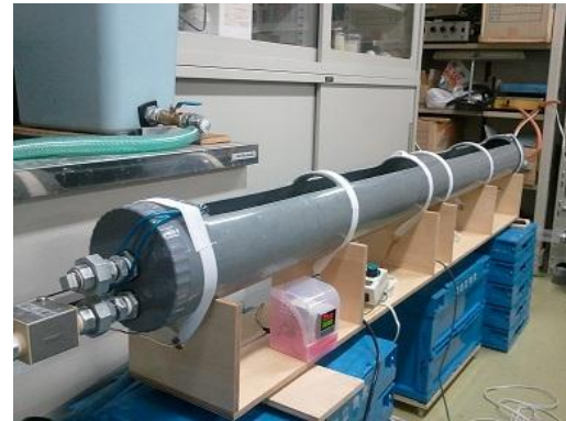
Fig.1 Photographic view of the open channel fluid flow experimental set-up.
