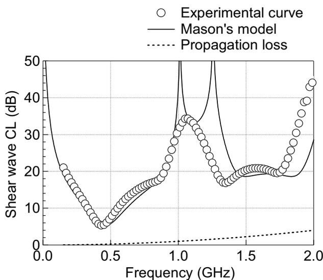
Fig. 2 Experimental and theoretical shear wave conversion loss of c-axis tilted ScAlN film resonator.
