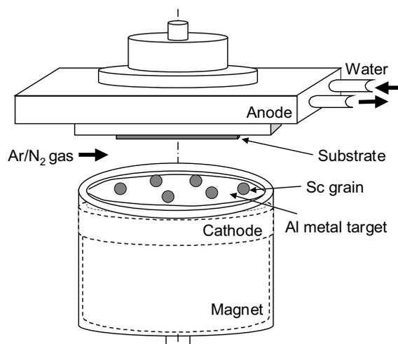
Fig. 1 Single planar RF magnetron sputtering system with Sc grain ingot on Al metal target.
