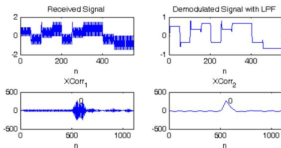
Fig. 5 Result of a DSSS Signal with Delay without Noise
