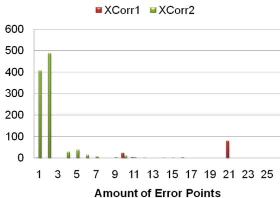
Fig. 7 Error Distribution of a DSSS Signal.
