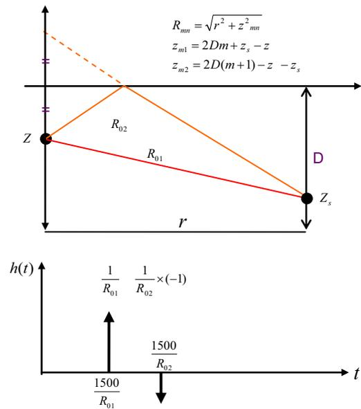
Fig. 3 Scheme of the Image Method.
