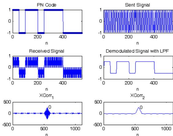
Fig. 4 Result of a DSSS Signal without Delay & Noise
