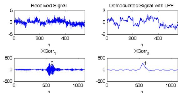
Fig. 6 Result of a DSSS Signal with Delay and Noise.
