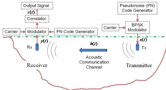
Fig. 1 Concepts of the Underwater Acoustic Communication Channel with DSSS system.
