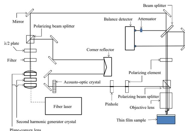
Fig. 1 Schematic of the optics. Solid and dashed lines represent laser beam with wavelength 532 nm and 1064 nm, respectively.
