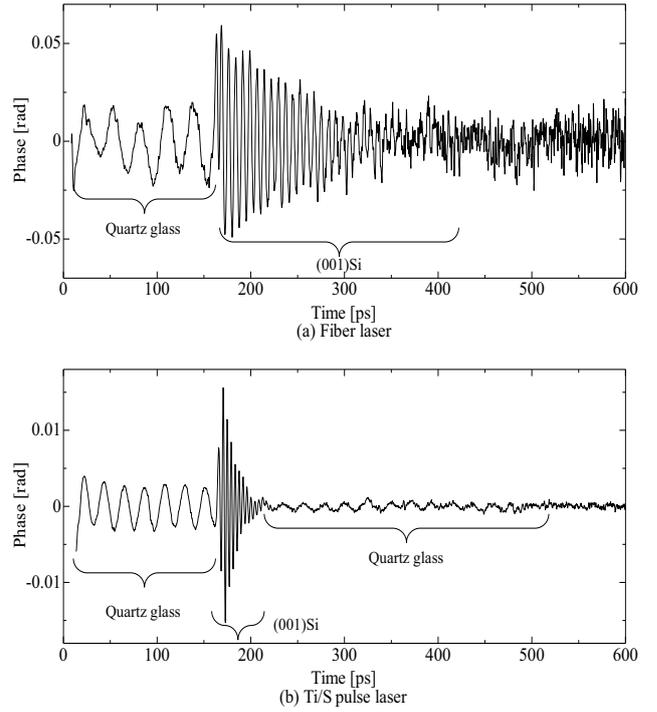
Fig. 3 Brillouin oscillations observed from SiO<sub>2</sub> thin film and Si substrate using PU systems incorporating (a) fiber laser and (b) Ti/S laser.
