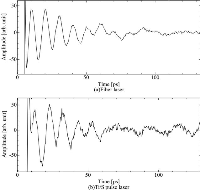
Fig. 2 Acoustic phonon resonance signals obtained from PU systems incorporating (a) fiber laser and (b) Ti/S laser.
