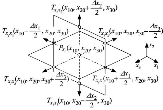
Fig. 2. A spatial grid of  $x_i$ -components of the momentum vector and the stress tensor at the point  $O(x_{10}, x_{20}, x_{30})$ .
