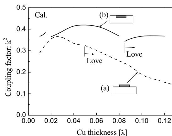
Fig.1 Electro-mechanical coupling factor on (a) conventional structure of Cu electrode on 4°YX-LiNbO<sub>3</sub> and (b) grooved Cu-electrode /4°YX-LiNbO<sub>3</sub>.
