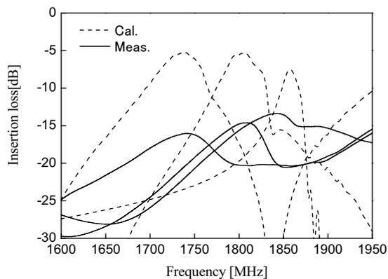
Fig.4 Frequency characteristics of band pass type tunable filter using Si diode variable capacitors.
