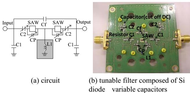
Fig.3 (a)Circuit and (b)PCB of tunable filter composed of Si diode variable capacitors and SAW resonators.
