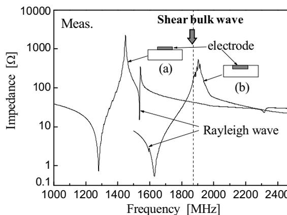
Fig.2 Frequency characteristics of SAW resonators composed of (a) and (b) structures in Fig. 1.
