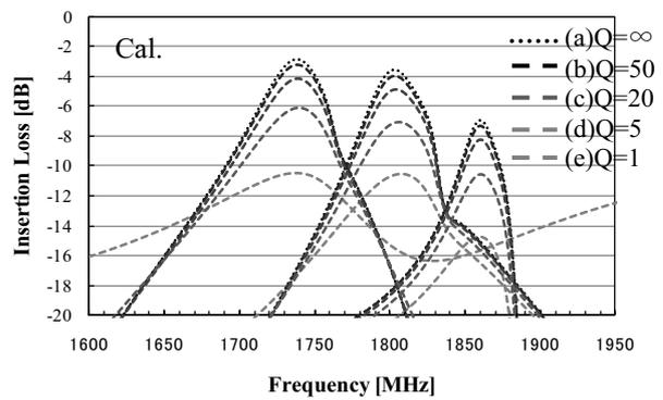
Fig.5 Calculated frequency characteristics on various  $Q$  value of variable capacitor
