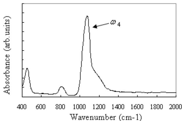
Fig. 1 FT-IR spectra of the deposited SiO<sub>2</sub> films
