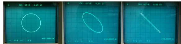
(a) a = b (b) a < b (c) a = 0, b \neq 0 Fig. 4 Circular /elliptic driving voltages based on Eqs. 1' transform relations.
