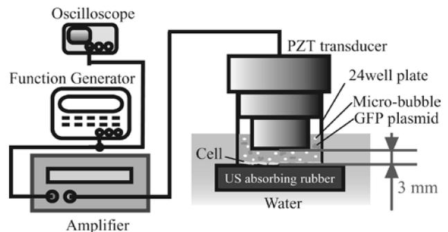
Fig.1 System setup
