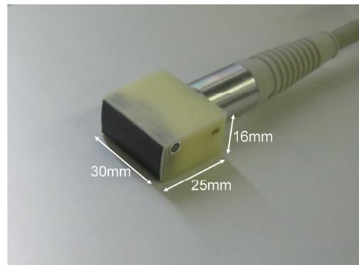
Fig. 1 Small prototype linear array
