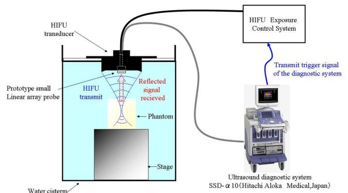
Fig. 2 Schematic of experimental setup in this study
