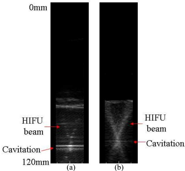
Fig. 4 Ultrasound images of the HIFU beam within the phantom;(a)3% agar phantom, (b)two layer agar phantom
