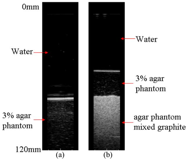
Fig. 3 Ultrasound images of the phantom; (a)3% agar phantom, (b)two layer agar phantom
