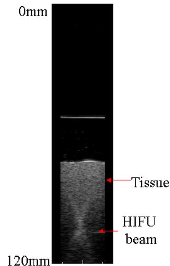
Fig. 5 Ultrasound image overlapped HIFU beam shape and the tissue for the two layer agar phantom
