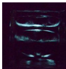
Fig.3 Sonoluminescence from glycerin and 80 % glycerin solution
