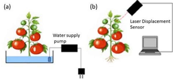
**Fig. 5.** Experimental setup for pseudo water stress to a plant. (a) Before the measurement: a tomato was raised by hydroponic culture, (b) On the measurement: water stress was given by cut the water supply off. The resonance frequency of a leaf was measured by a laser displacement sensor.
