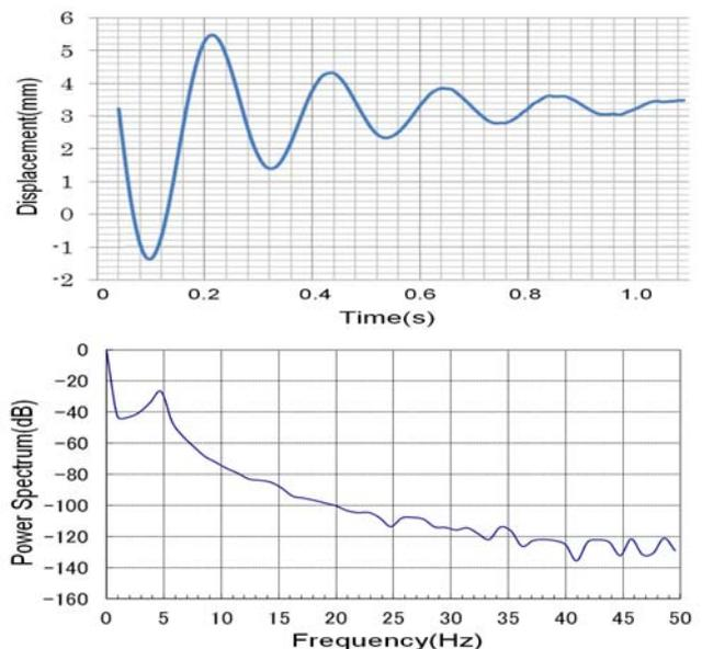
Fig. 2. A typical example of measurement result of the vibration of a leaf by a laser displacement sensor. (a) Vibration displacement, (b) Frequency analysis result.
