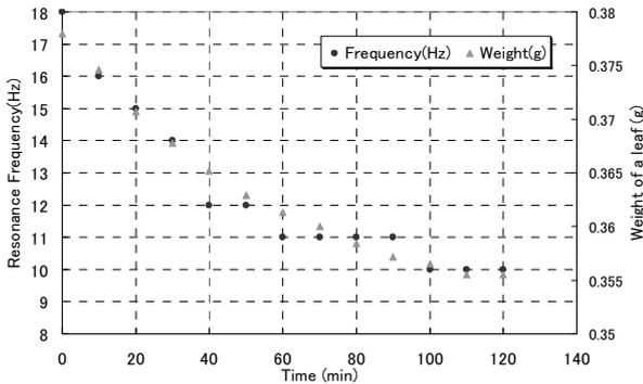
**Fig. 3.** The temporal change of the resonance frequency and the weight of a leaf. gray triangle: the temporal change of a leaf weight, black circle: temporal change of the resonance frequency.
