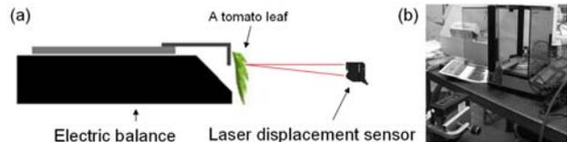
Fig. 1. An experimental setup using a cut leaf. (a) Schematic view of the experimental setup, (b) Photograph of actual experimental setup.
