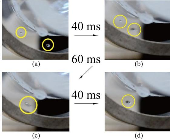
Fig. 3 Process of droplet mixing: photos of (a), droplets levitated at different nodes; (b), droplets moved by the modulated sound field intensity; (c), droplets that have begun to mix induced by surface tension; and (d), a mixed droplet.
