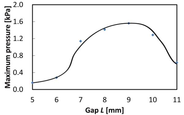
Fig. 5 Maximum sound pressure vs. gap between the vibration ring and the reflector.
