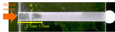
Fig. 4 Behavior of liquid in the pore (liquid surface : 5.5 mm)
