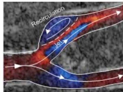
**Fig. 2** CESI screenshot when imaging a bifurcation with stenosis at the inlet to upper branch. Flow directions and key flow events have been labeled.
