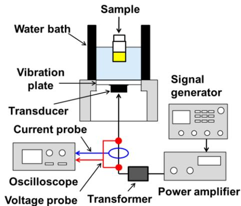
Fig.2 Experimental setup
