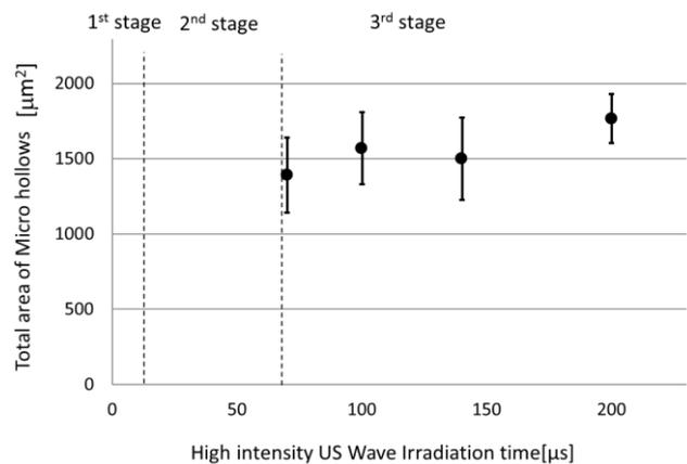
Fig.4 Total area of micro hollows for different irradiation time of ultrasonic wave
