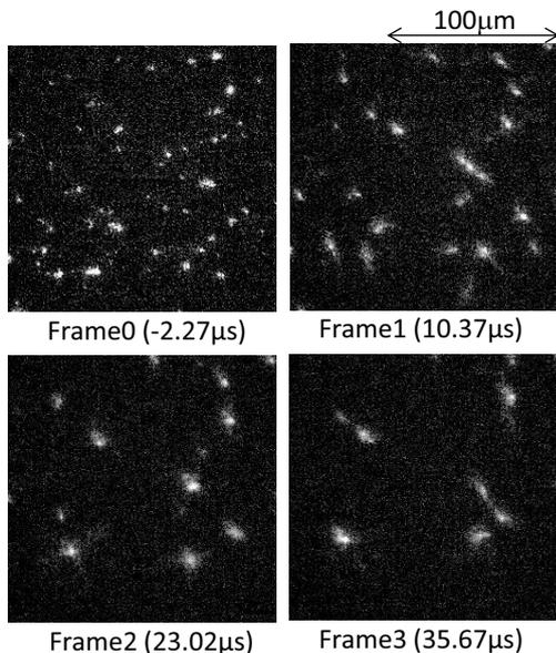
Fig2 Photographs of bubble clouds when high intensity US wave irradiates
