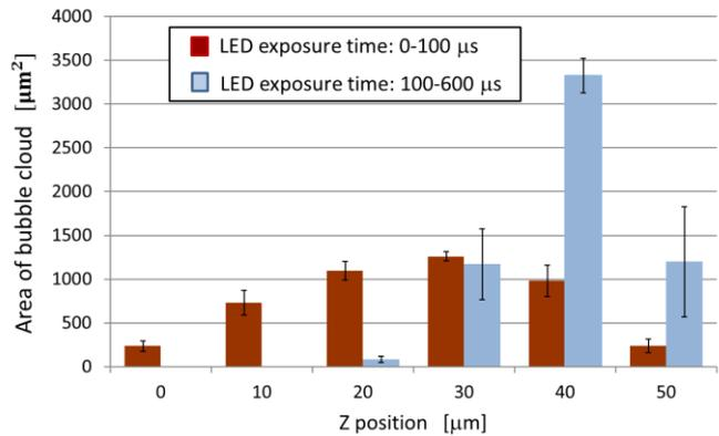
Fig.3 Measurement of Z-position of bubble clouds
