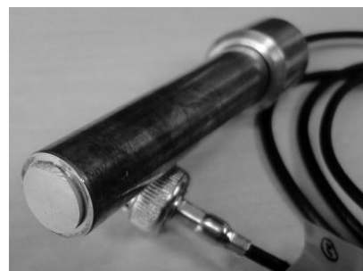
Fig. 2 An example of bone transducer.
