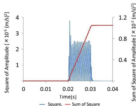
**Fig. 1.** An example of the amplitude square of a received waveform (blue line), and grand total of the amplitude square (red solid line).
