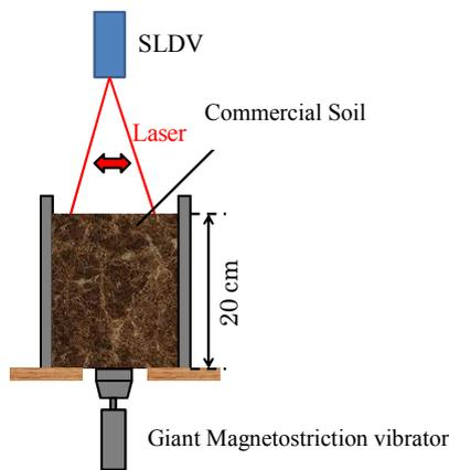
Fig. 2. Experimental setup for propagation velocity.
