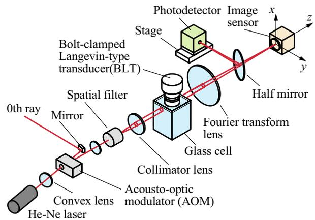
Fig. 1 Schematics of experimental system.
