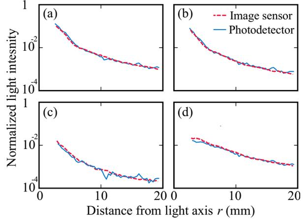
Fig. 3 Diffraction pattern in radial direction.
