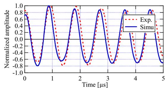
Fig. 2 Waveforms of experiment and simulation at focal point in sound field.
