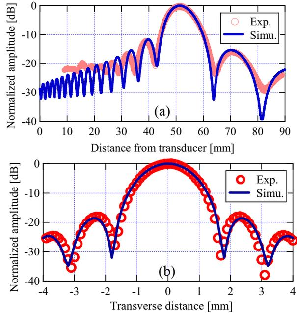
Fig. 1 Sound pressure distributions of experiment and simulation, (a) at central axis, (b) transverse direction on focal point.
