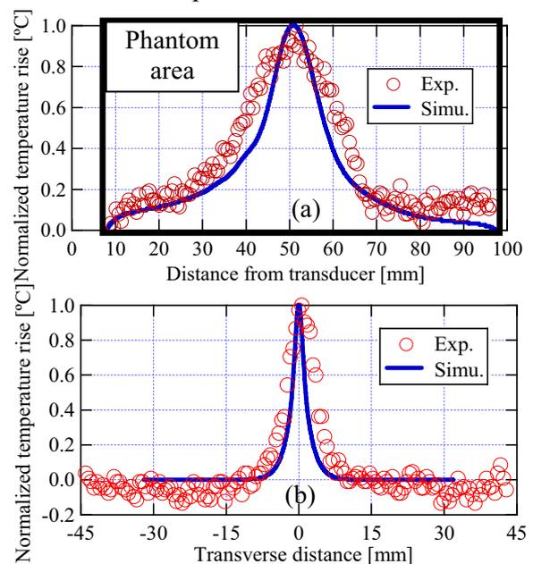
Fig. 3 Temperature rise distribution of experiment and simulation, (a) at central axis, (b) transverse direction on peak temperature rise point.
