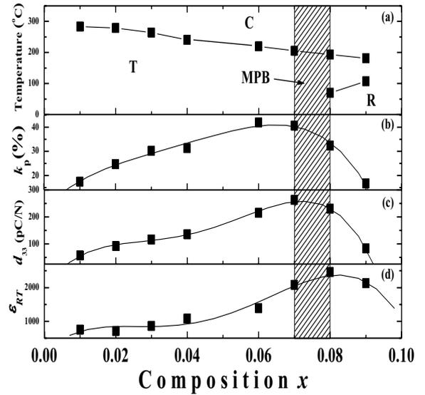
Fig. 3, (a) Phase diagram, and (b),(c),(d) composition dependence of dielectric and piezoelectric properties.
