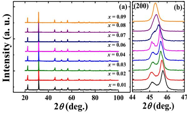
Fig. 1, (a) XRD patterns at room temperature; (b) Pseudo (200) reflection peaks for  $0.90(\text{Na}_{0.5}\text{K}_{0.5})\text{NbO}_3-x\text{BaZrO}_3-(0.10-x)(\text{Bi}_{0.5}\text{Li}_{0.5})\text{TiO}_3$  ceramics.
