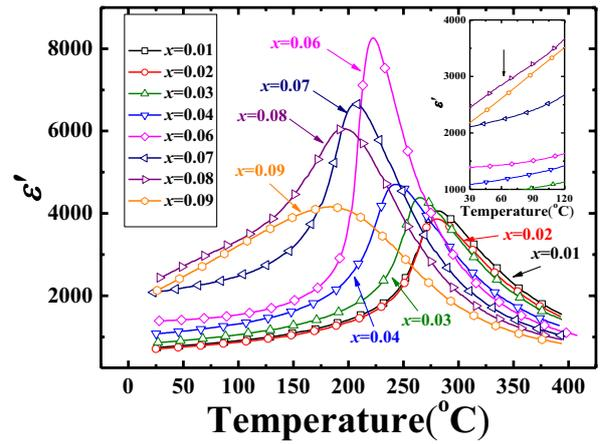
Fig. 2, The temperature dependence of the dielectric constant for  $0.90(\text{Na}_{0.5}\text{K}_{0.5})\text{NbO}_3-x\text{BaZrO}_3-(0.10-x)(\text{Bi}_{0.5}\text{Li}_{0.5})\text{TiO}_3$  ceramics.
