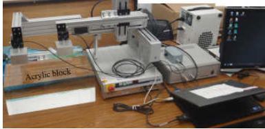
Fig.2 System of non contact air coupled ultrasonic inspection (V-Transmission method)
