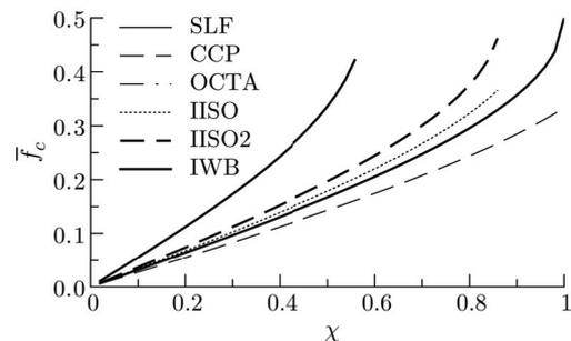
Fig. 2 Cut-off frequency against CFL number.
