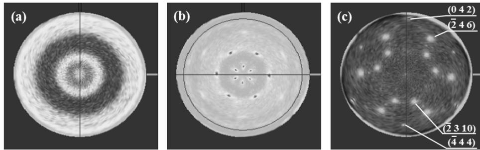
Fig. 2 Pole figures of (a)  $\text{Ta}_2\text{O}_5/\text{SiO}_2$ , (b)  $\text{Ta}_2\text{O}_5/c\text{-Al}_2\text{O}_3$  (no pretreatment), and (c)  $c\text{-Al}_2\text{O}_3$ .
