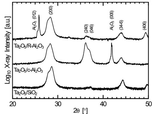
Fig. 1 XRD patterns of Ta<sub>2</sub>O<sub>5</sub> thin films deposited on *R*-Al<sub>2</sub>O<sub>3</sub>, *c*-Al<sub>2</sub>O<sub>3</sub> (no pretreatment), and SiO<sub>2</sub>.
