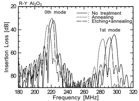
Fig. 3 Frequency responses of IDT/ $\text{Ta}_2\text{O}_5/\text{R-Y Al}_2\text{O}_3$  samples.
