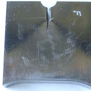
Fig. 2 Cut-out sample with a fatigue before surface grinding.
