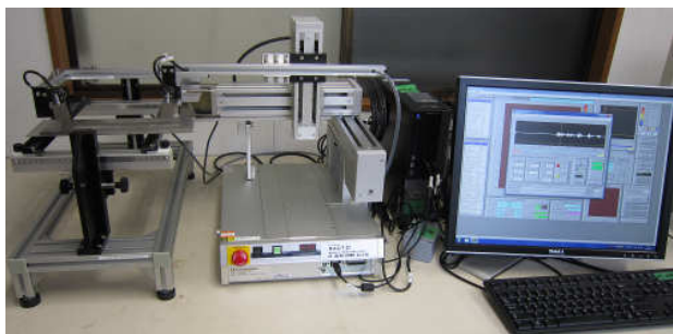
Fig.3 System of non contact air coupled ultrasonic inspection (Lamb wave method)
