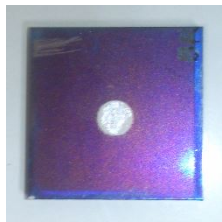
Fig.1 BiT/PZT film optical images made by stencil printing onto \sim 3\text{mm} thick titanium substrate.
