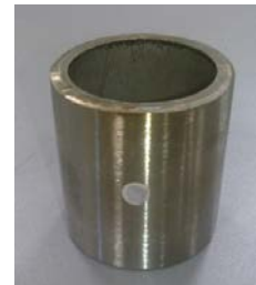
Fig.4 BiT/PZT film optical images made by stencil printing onto \sim 40\text{mm} outer diameter steel pipe.
