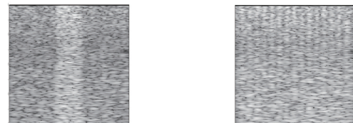
(a) Fiber width: 8mm (b) Fiber width: 0.53mm Fig. 2 B mode image of scatterer
