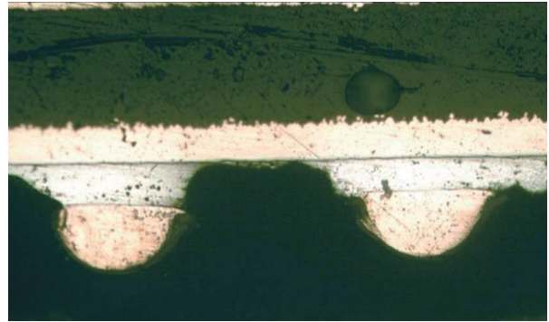
Fig. 3 The cross-sectional OM image of Cu electrode and Cu bump joint with Sn-58Bi solder
