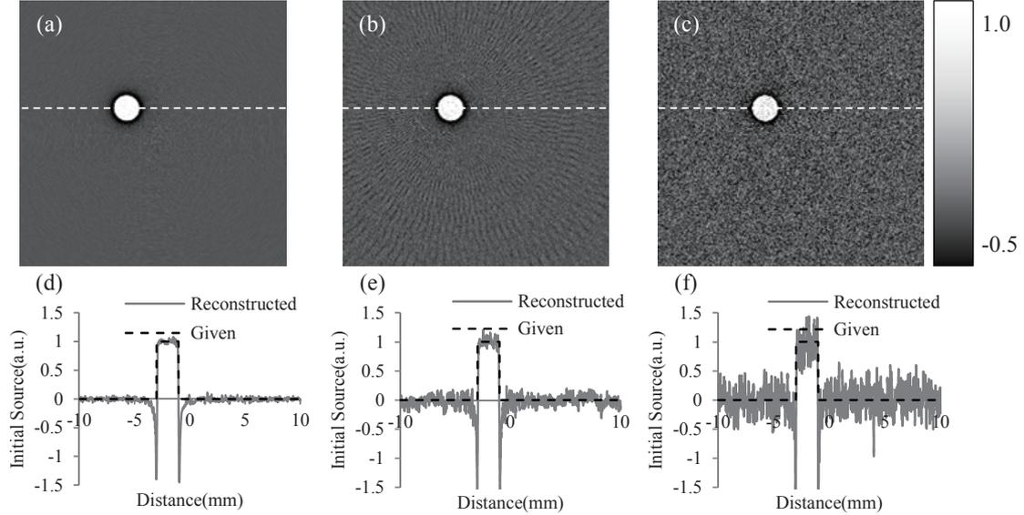
Fig. 2 Reconstructed images (a-c) and profile of initial source along broken line (d-f); (a), (d) using coded excitation and changing start point of decoding, (b), (e) using conventional coded excitation, and (c), (f) using continuous data acquisition method.
