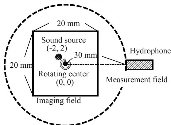
Fig. 1 Simulation setup for PACT.
