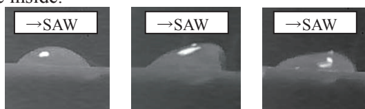
Fig. 1 : Droplet manipulation by SAW.
