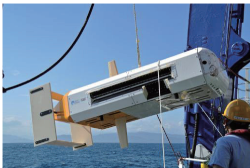
Fig. 1 The tow-fish specially made for the Synthetic Aperture Sonar.
