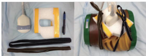
Fig. 1 Left image shows 3D probe, hand-made probe holder using polyurethane foams, and bands for fixation. Right image shows the fixed probe on a body phantom.
