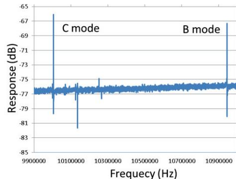
Fig. 2 Frequency characteristics of the SC cut resonators
