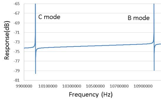
Fig. 6 The SC cut resonator by the simulation
