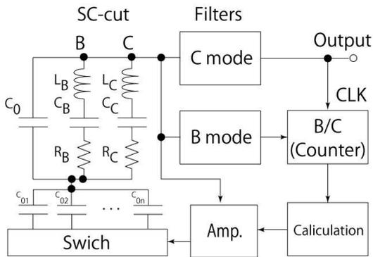
Fig. 4 Block diagram using the SC cut resonator
