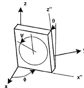
Fig. 1 Azimuth of the SC cut resonator<sup>[4]</sup>
