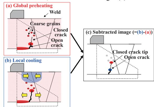
Fig. 1 Schematic illustration of GPLC and LDPA.
