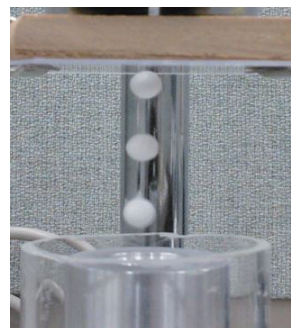
Fig. 1 Experimental results of ultrasonic levitation using Langevin transducer at 20.5 kHz.
