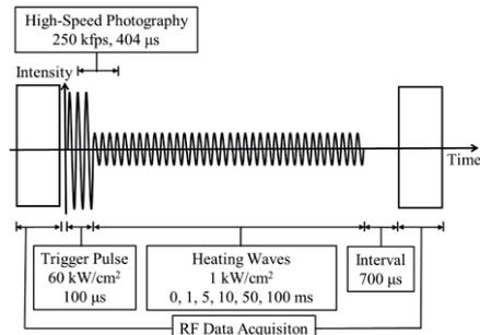
Fig. 2 Sequence of HIFU exposure and RF data acquisition
