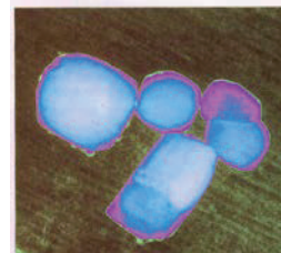
Fig.1. Diamond crystallites grown by sputtering process at room temperature. Size of crystallites, \sim 0.1\mu\text{m} . Sputtering, ion beam sputtering [2].
