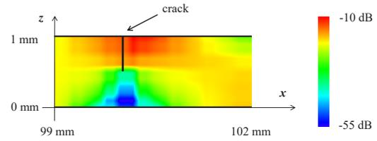
**Fig.3** Computer simulation result of acoustic field of second harmonic components in a plate near a crack using finite element method.
