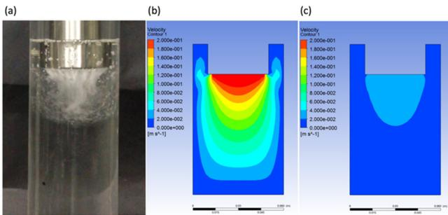
Fig. 1. (a) Experimental results, (b) the modeling of calculation attenuation factor and (c) after correction
