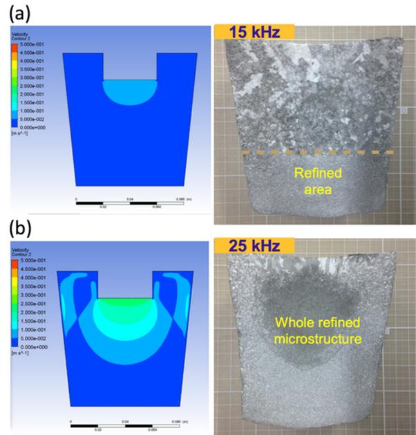
Fig. 2. Comparing of ANSYS simulation result by the revised attenuation factor with castings of A356; (a) 15 kHz and (b) 25 kHz.
