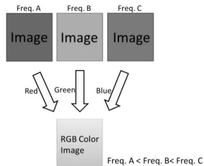
Fig. 2. Concept of multispectral phase-contrast imaging.
