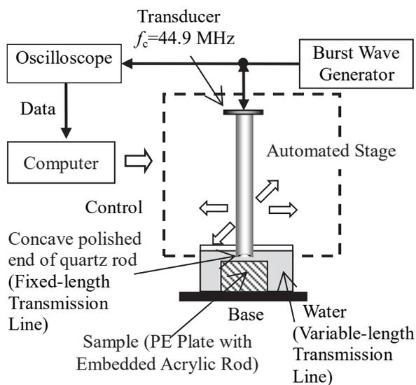
Fig. 3. Schematic diagram of experiment.
