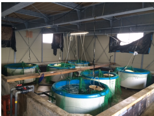
Fig. 2. Six FRP 1.0 m 3 water tanks used for S&LIPUSS for Sakura masu experiment in a warehouse.
