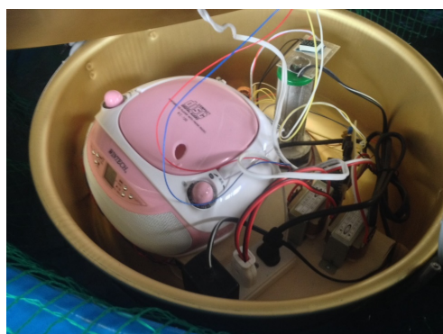
Fig. 4. The S&LIPUSS equipment with a music speaker, 350 Hz sound and four of 500 kHz PZT transducers used for #3 tanks.
