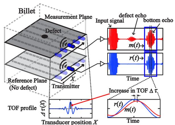
Fig. 1 Outline of defect detection by time-of-flight deviation of bottom echo.<sup>3)</sup>
