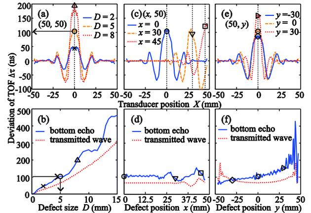
Fig. 3 Deviation of TOF  $\Delta\tau$  when the defect size  $D$  or position  $(x, y)$  are varied: (a) TOF profile at the  $D = 2, 5, 8$  mm, (b) relationship between  $D$  and  $\Delta\tau$ , (c) TOF profile at  $x = 0, 30, 45$  and  $y = 50$ , (d) relationship between  $x$  and  $\Delta\tau$ , (e) TOF profile at  $x = 50$  and  $y = -30, 0, 30$ , and (f) relationship between  $y$  and  $\Delta\tau$ .
