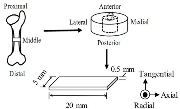
Fig. 1 Preparation of samples.
