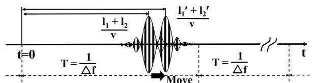
Fig. 3 Impulse responses calculated by IFFT and subtraction between two impulse responses for Fig. 1's model.
