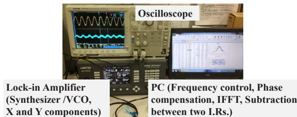
Fig. 5 Developed automatic-measurement system at 18-19 kHz (Subtracted data are stored in PC).
