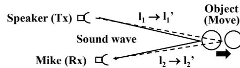
Fig. 1 Transmission and reception of sound waves at upper vocal register via reflecting object.
