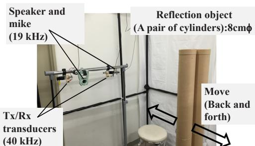
Fig. 6 Experimental setup. A pair of cylinders with 8 cm $\phi$  can move. Speaker and mike around 19 kHz are fixed at about 1.5-m height. Tx and Rx transducers at 40 kHz are also fixed for comparison.
