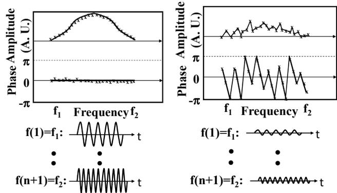
(a) Transmitted signals (b) Received signals
