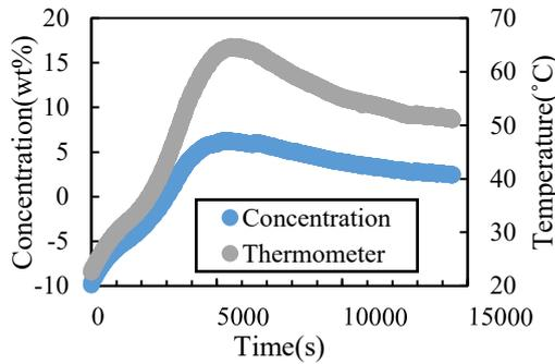
Fig. 3 Estimated methanol concentration.
